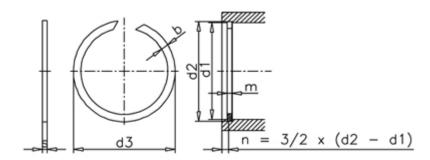
$\begin{array}{lll} b & = 7.50 \\ d1 & = 370 \\ d2 & = 375.0 \\ d3 & = 378.5 \\ Description = SB 370 \\ FN kN & = 493.00 \\ FR kN & = 116.00 \\ m min & = 4.2 \\ \end{array}$
